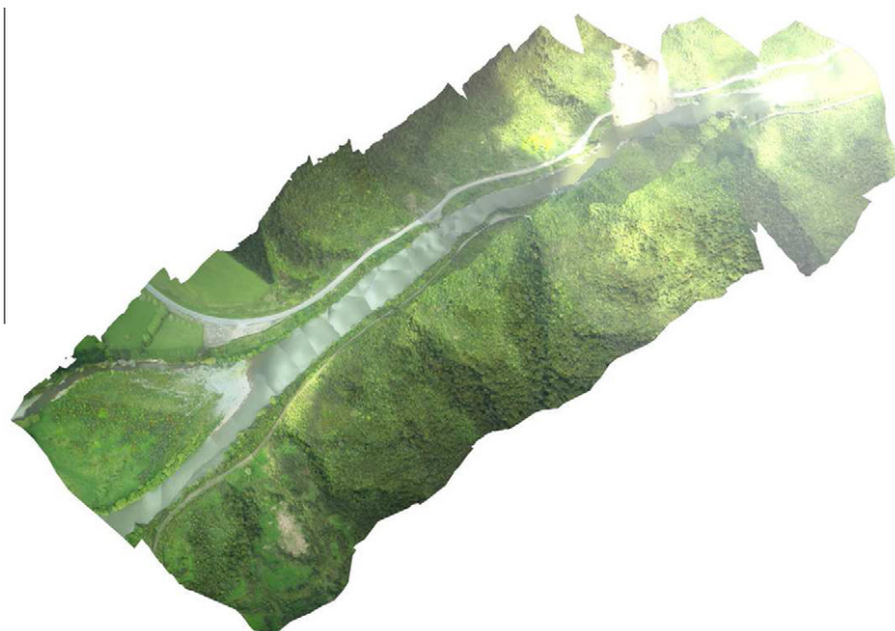
Fig. 18. Final mosaic for the Manawatu data set using Optimal vertex placement (Method 3).
