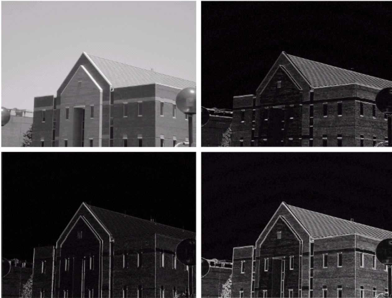
FIGURE 10.10 (a) Original image. (b) |G_x| , component of the gradient in the x -direction. (c) |G_y| , component in the y -direction. (d) Gradient image, |G_x| + |G_y| .
