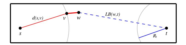
Reach-based query algorithm is Dijkstra's algorithm with pruning based on reaches. Given a lower-bound subroutine, a small change to Dijkstra's algorithm.
